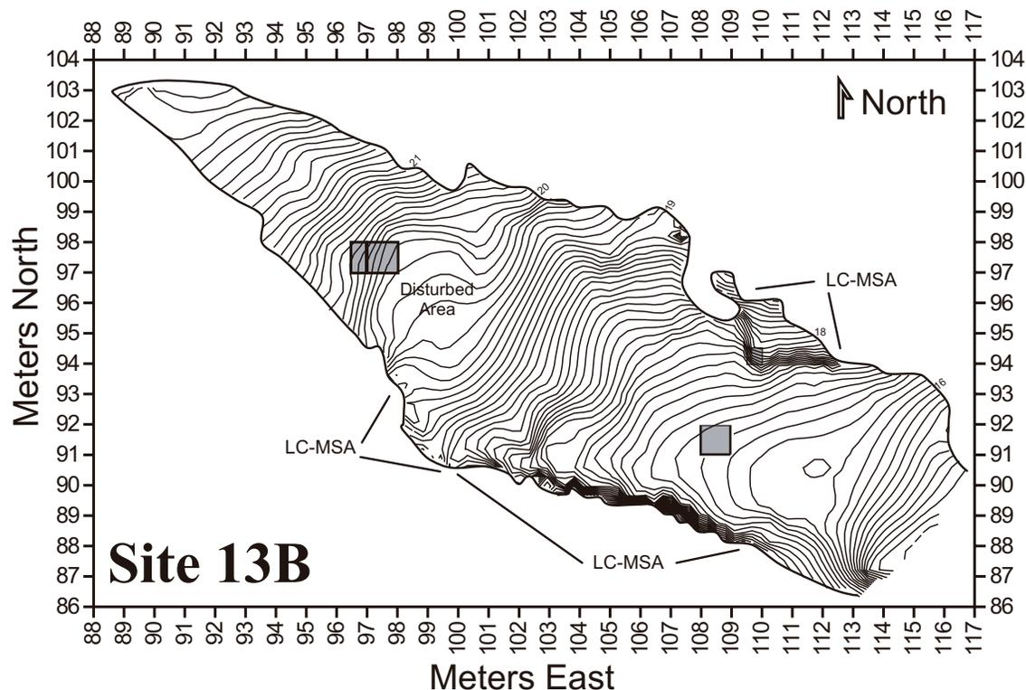
Figure 14. The outline and topography of Site 13B, and the position of the test pits (the grey boxes). The contours are in meters asl, at 10 cm increments. LC-MSA is the lightly consolidated MSA deposits. Orientation is magnetic north.
